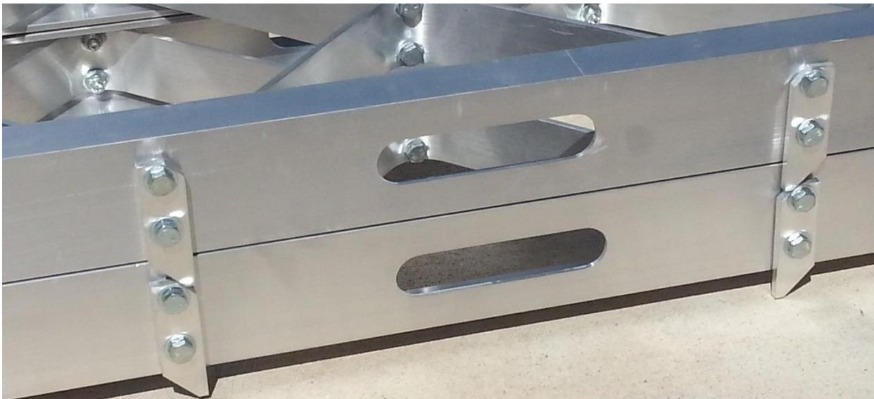
Torque all bolts to 20 ft-lbs, starting in the center and working out to the ends. Check the torque of the bolts after the first use of the bridging ladders and after every several uses thereafter.
