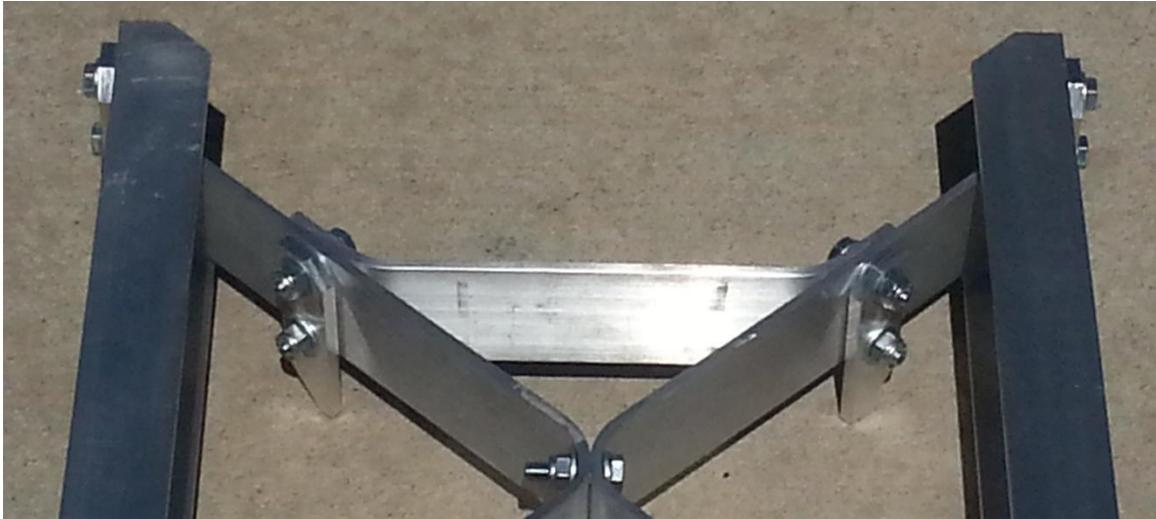
Once all the pieces have been loosely assembled snug the bolts up to eliminate any play, starting at the center of the bridging ladder and working out to the ends. Snug up the bolts for the End Treads last. Stack the two bridging ladders together and check the alignment of the Grip Cleats. The Cleats on the top and bottom ladders should be in alignment as shown below.
