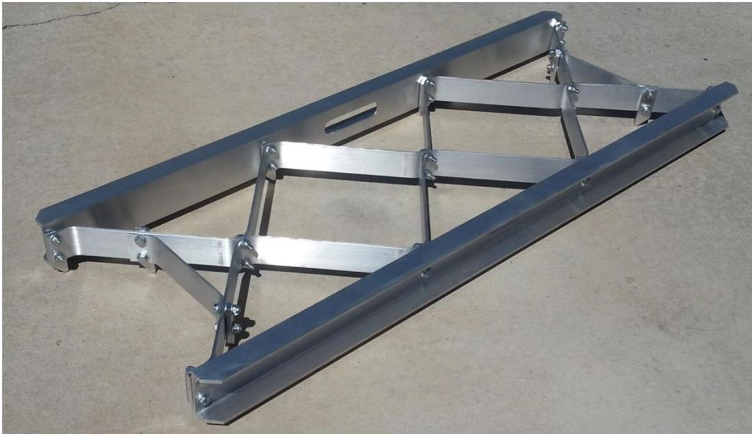
Decide on the assembly option to use and then loosely assemble the parts together, always using a washer under the bolt head and nut. The Grip Cleats should always be positioned so the large chamfer faces toward the ends of the ladder. This means the Cleats on one half of the ladder will face one way, and the other half will face the other way.
